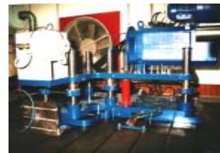
X-Y-Z positioner unit with 7-pillar guide for the mounting of a driving unit
