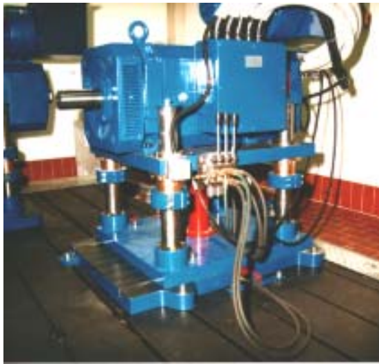
X-Y-Z positioner unit with 4-pillar guide for the mounting of a braking unit
